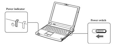
If you hold the power switch in the On position for more than four seconds, the computer turns off.
